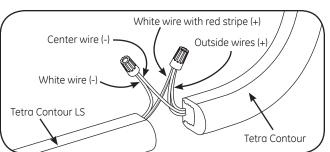
2 Splice the white wire with red stripe (+) of Tetra Contour LS to the two outside wires (+) of Tetra Contour and splice the white wire (-) of Tetra Contour LS to the center wire (-) of Tetra Contour. Insert wire connectors into weather box. Fill with electrical grade silicone and close box.
