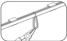
If required, cut wire loops between sections or through light engine in the appropriate area (refer to the Cutting Resolution table above).
