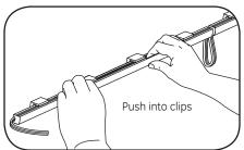
Push each 16 in. (406mm) light engine segment into the clips. Fold loose wires behind light engines.
