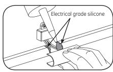
8 At each gap between Tetra Contour sections, snap on a light guide connector.
