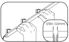
Attach Tetra Contour to the mounting clips, leaving a 3/8 in. (10mm) gap between sections to allow for expansion or contraction. Secure light guide by twisting tie-wire around the mounting clip and light guide.
