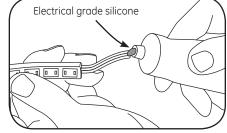
6 CAUTION: Anytime light engine or supply wire is cut and/or wire is exposed, electrical grade silicone must be applied (see list on the next page for recommendations).
