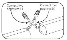
Use twist-on wire connectors to join wires together. Fold wires behind light engines.
