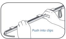
Push each 16 in. (406mm) light engine segment into the clips. Fold loose wires behind light engines. Do not stretch light engines.
