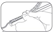
Push the light engine segments down into the light guide.
