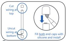
For vertical or near vertical installations, any cut-end termination of a Contour piece shall reside at the top of the design.
