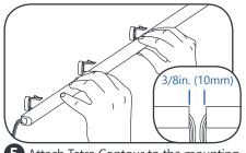
5 Attach Tetra Contour to the mounting clips, leaving a 3/8 in. (10mm) gap between sections to allow for expansion or contraction.
