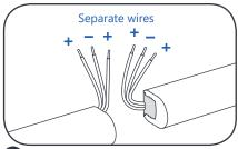
8 To connect two light engines separate wires and identify outer conductors as positive (+) and middle conductors as negative (-). Strip ends back 0.5 in. (13mm).
