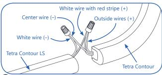
Splice the white wire with red stripe (+) of Tetra Contour LS to the two outside wires (+) of Tetra Contour and splice the white wire (-) of Tetra Contour LS to the center wire (-) of Tetra Contour.
