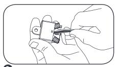
3 Insert wire connectors into weather box. Fill with electrical grade silicone and close box.
