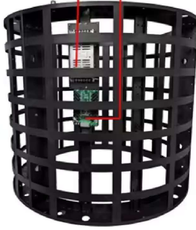
Install receiving card and power supply
